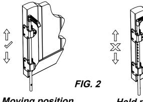
**Moving position**Rod is free to move up or down when lock cylinder is in unlocked position
