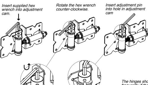
Carefully rotate the adjustment cam clockwise until the adjustment pin contacts the fence post leaf. Remove the hex wrench. Repeat until gate closes firmly.
