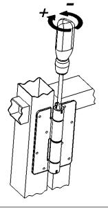
The hinge should be inspected annually, or more frequently if the gate is used often. Spring tension adjustments should be made as needed. The hinge should be regularly lubricated by spraying an oil based lubricant into the area of the cams and barrel.
