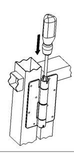
and counter-clockwise to reduce spring tension. Adjust one hinge at a time in 1/4 turn increments.
