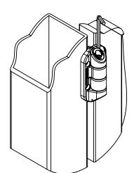
Rotate the cam clockwise to increase (+) spring tension. To decrease (-) spring tension, press the wrench downward, pushing the cam into the barrel, and rotate the cam counterclockwise. Adjust one hinge at a time in 1/4 turn increments.
