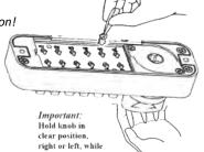
While holding the thumb-turn, remove/add CODE (Red) and NON-CODE (Blue) Tumblers to create your desired code.
