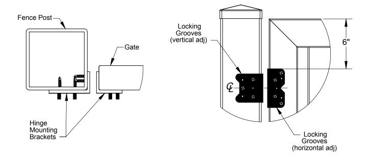
Install self closing hinge assembly to mounting brackets (installed in step 1) and secure with acorn nuts (USE HAND TOOLS ONLY). Hinge should be positioned as shown so that the locking grooves on the mounting flanges will align with grooves on the back side of the hinge assembly. This will allow the hinge to be adjusted horizonally on the gate side, and vertically on the post side.
